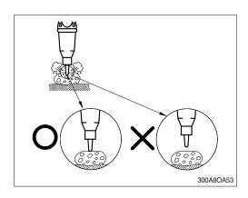
Move the impact point from the edge to the interior. Never try to break off a too large block, if the object has not broken within 30 seconds. The object should be broken up piece by piece in small blocks. Large distance steps will not improve working results.
