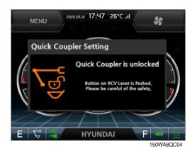
(7) Retract the bucket cylinder. Align the quick coupler with attachment mounting pins or interface.
