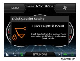
(5) To unlock the quick coupler, press the quick coupler button on the right RCV lever.
